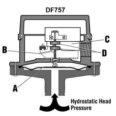
For reference only, DF757 is not available. The DF757 trip point is adjustable over a 108 in. (2743 mm) differential.
