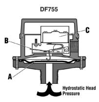
The SPDT snap-switch for the DF755 is preset for a 4 in. (102 mm) differential in liquid level.
